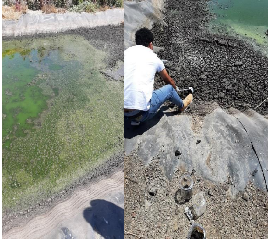
Figure 3.2: Sludge sampling from the drying beds
