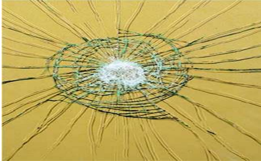
Figure2.6: The interlayer holds the broken glass fragments in laminated glass (Tom castle, 2012)
