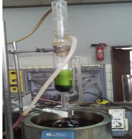
Fig 3.3-1 Extraction processes of WH Extractives
