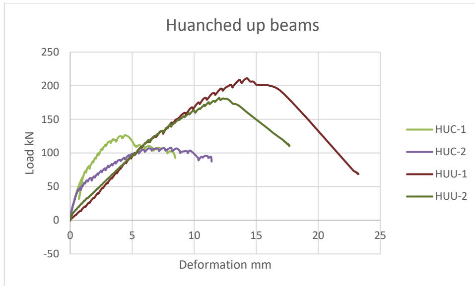
Figure 5-5: Load deformation diagram of haunched up specimens
