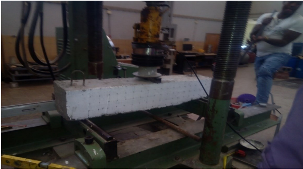
Figure 4-6: Test set up for concentrated load test
