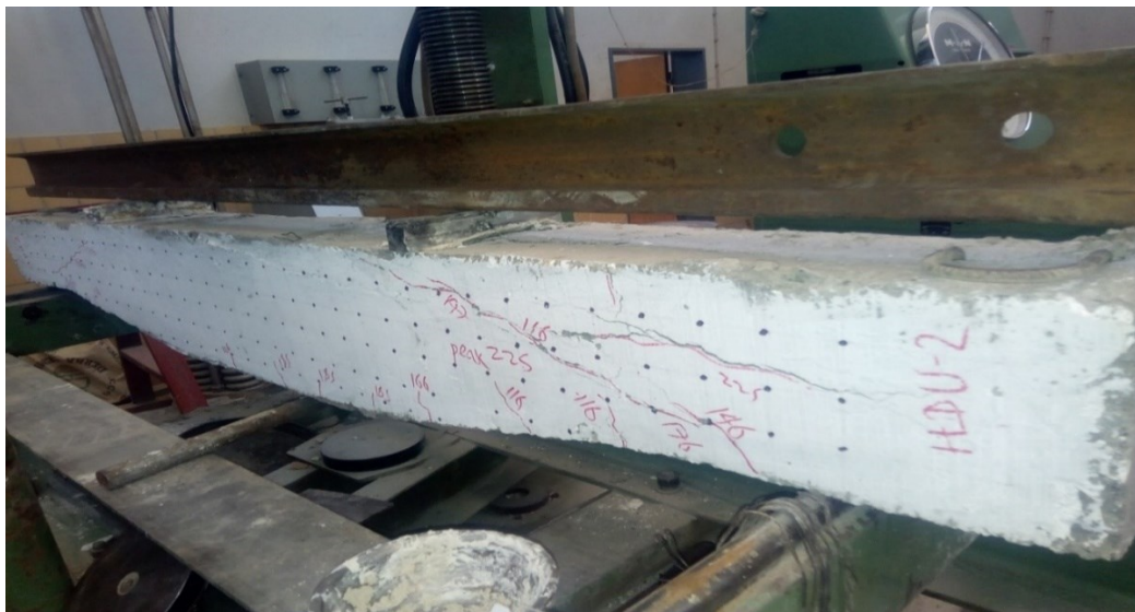
Figure 4-7: Test set up for uniformly distributed (two-point load) load test
