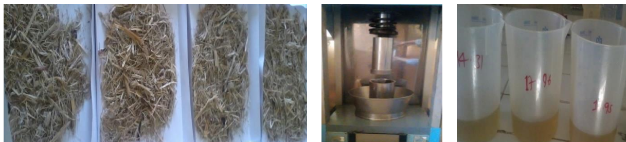
(a) Prepared sucrose free fiber (b) Hydraulic press (c) 10° Brix sucrose solution
