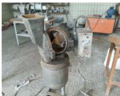
Figure 10: Coffee husk grinding and sieving
