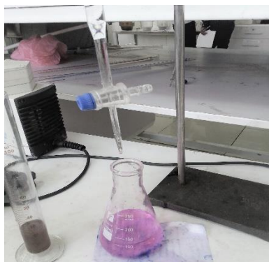
Figure 24: Titration of Acetic acid with 0.5M NaOH
