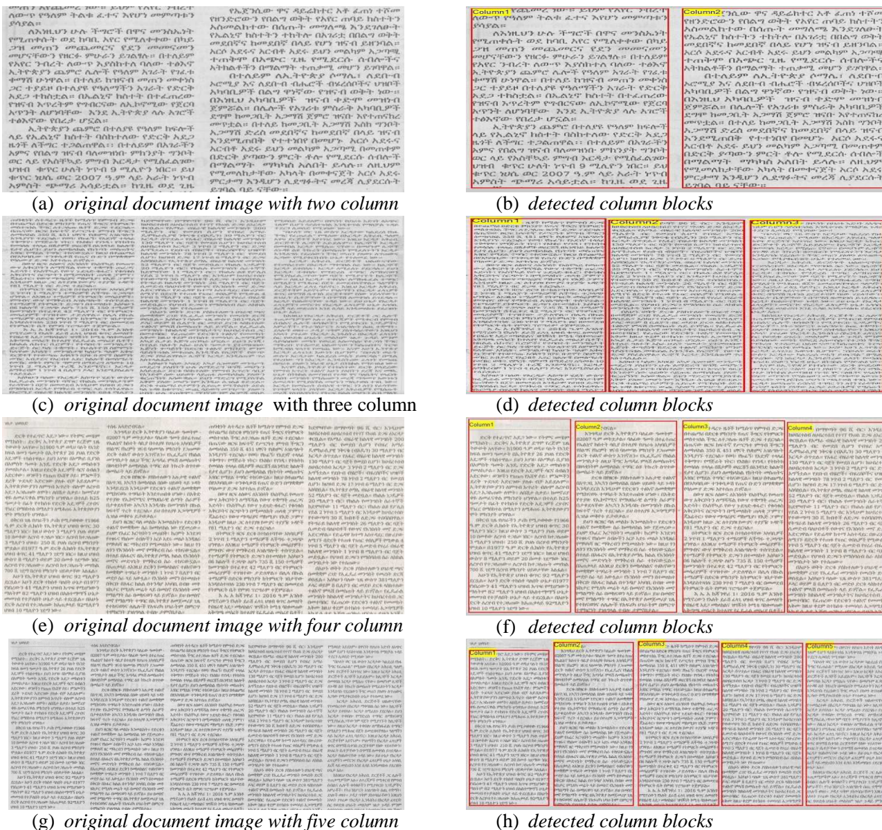
Figure 4.5: Experimental result after the proposed column block segmentation techniques applied
