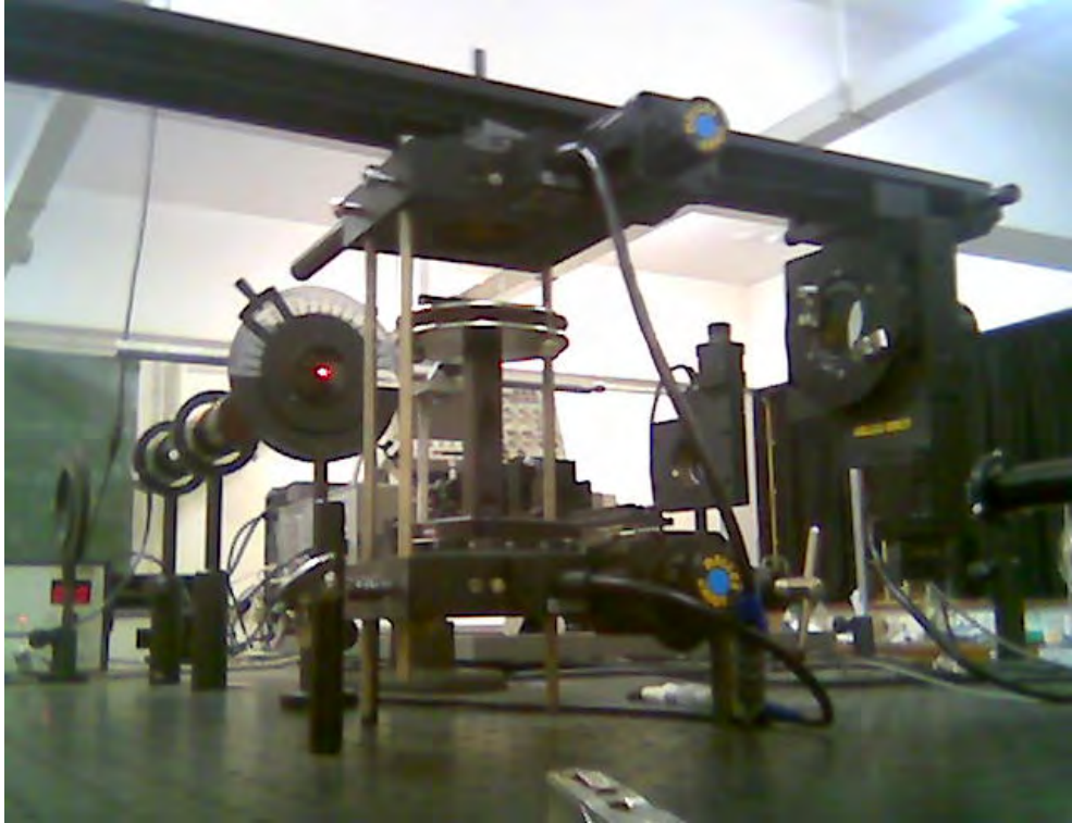
Figure 3.2: Automated ellipsometer setup.
