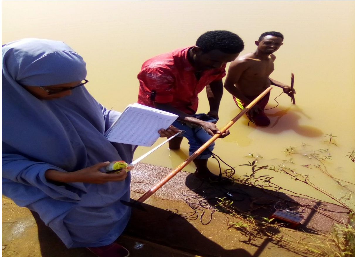
Figure 3-4: Calibration of the sounding instrument at koga night storage reservoir
