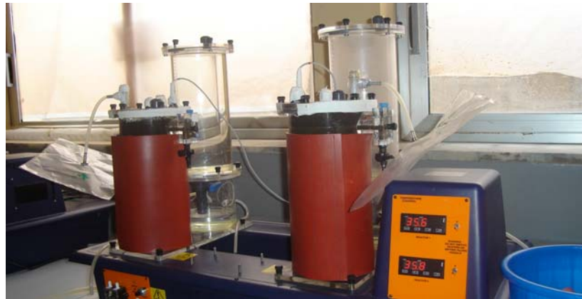
Figure 3.1: Anaerobic digester used during the test run
