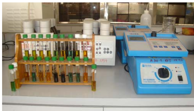
Figure 4.1 Test tubes after test, COD and BOD measuring instrument used in the study.
