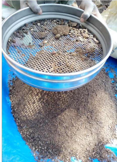
Figure 3-11: Preparation of sand for specimen preparation
