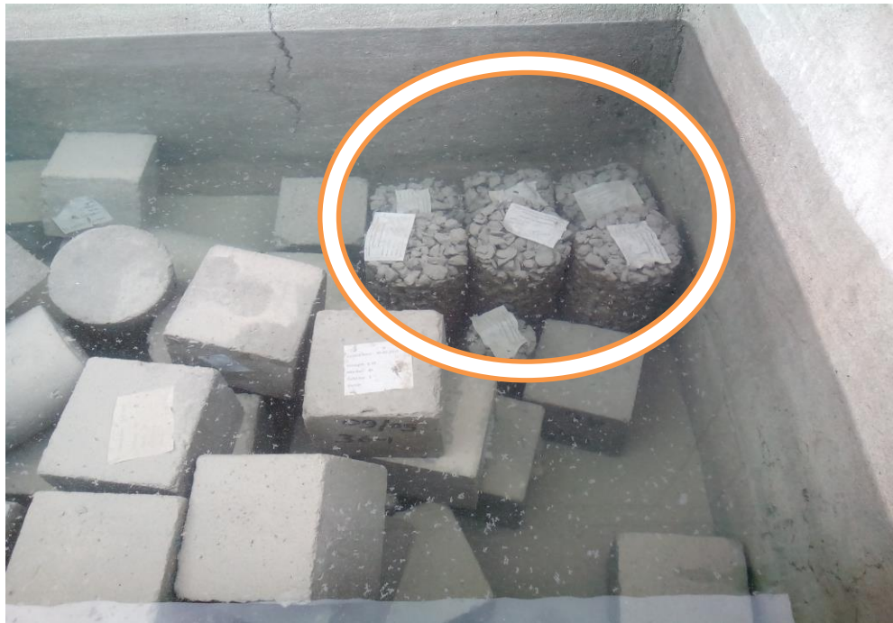
Figure 3-15: Specimens inside a curing bath
