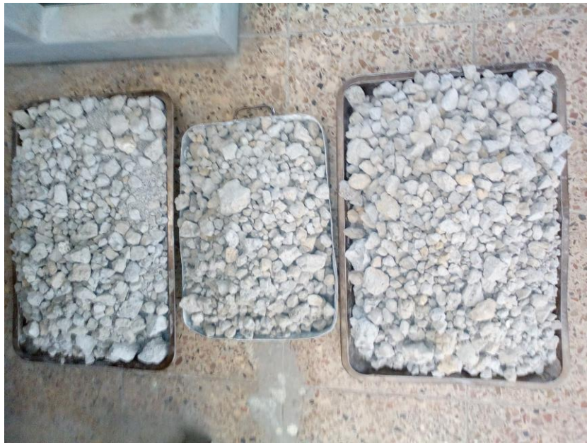
Figure 3-9: Air dried Pumice stone ready for grinding
