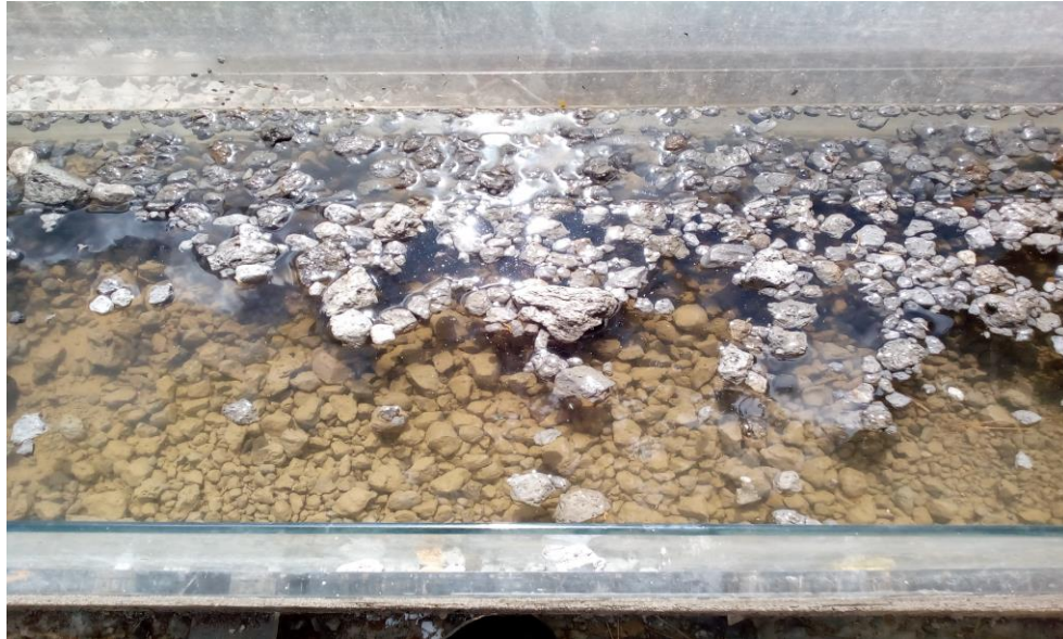
Figure 3-4: Volcanic pumice aggregates floating on laboratory water bath (Photograph courtesy of Abel W.)
