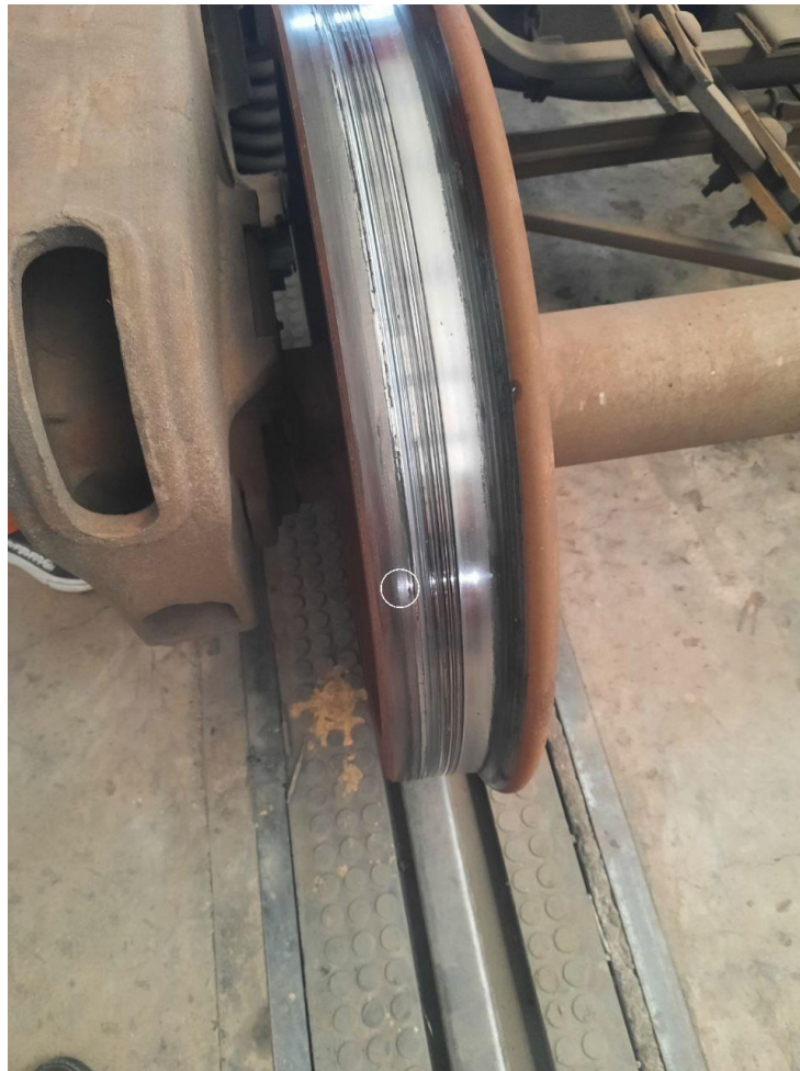
Figure 6: Defect occurred on EDR Train wheels with a small wheel flat
