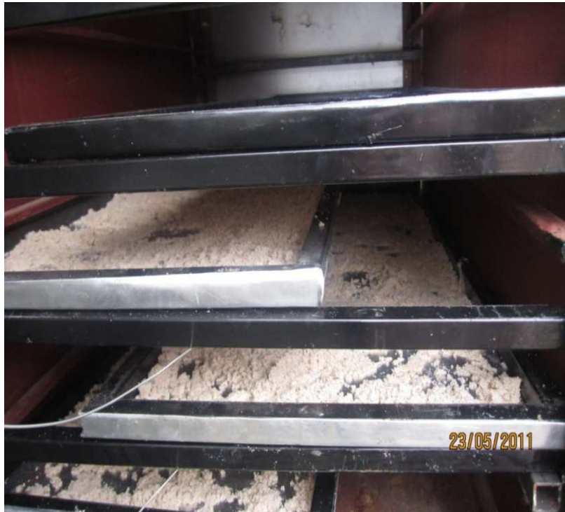
Figure 7.3 Picture Which Shows How Trays Were Placed in Drying Chamber
