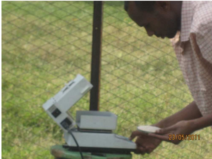
Figure B-1 Shows Mass Balance of Silica Sand during Experiment.
