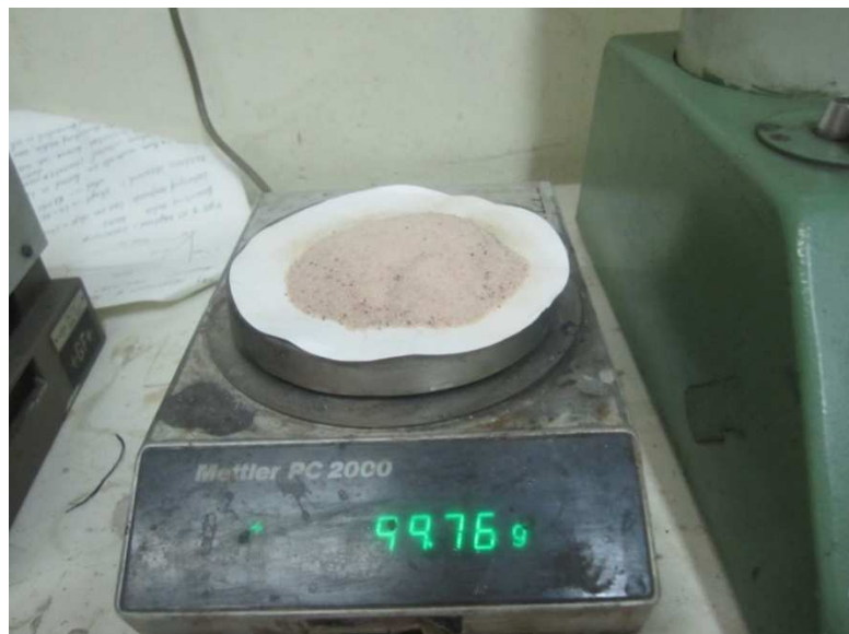
Figure 3.4 Moisture Balance for Silica Sand Dry Basis.
