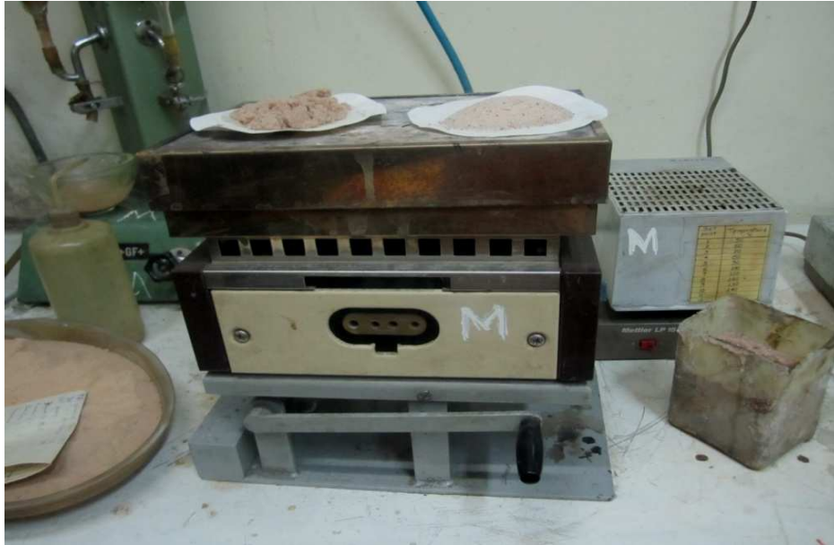
Figure.5.2 determination of moisture content of silica sand experimentally
