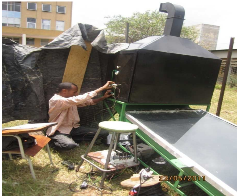
Figure B-3 Sensor Positioning to Take Reading Experimentally
