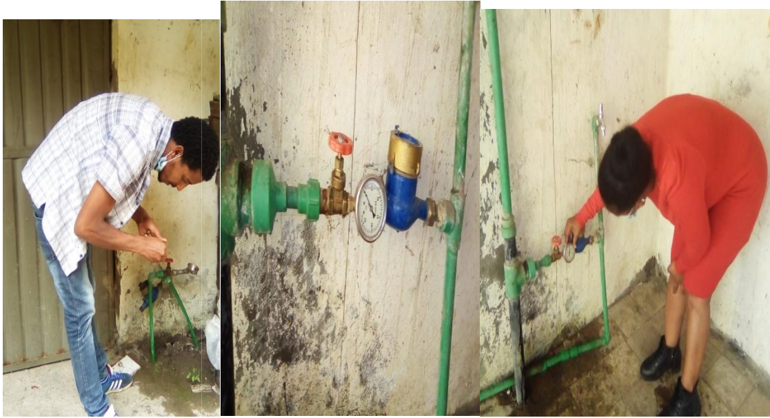
Figure 3.8 Pressure reading measurement using pressure gauges
