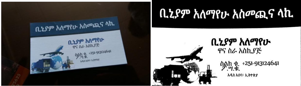
Figure 4.11: Example image of white texts on a dark background (a) Original document Image (b) Binarized and skew corrected document image
