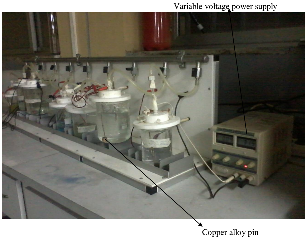
Figure 20: specimen in corrosion studies kit
