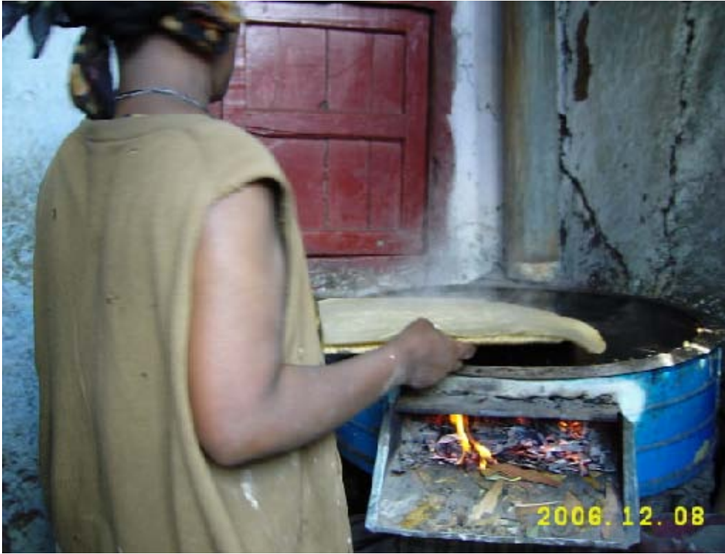
Plate 2. woman bakes 'injera' with modified traditional stove(Lakech mitad) . The fixed 'laketch stove is located on the veranda.
