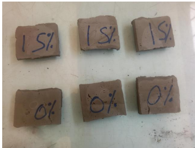
Figure 3.11. Samples Prepared for Bound Water Determination Test
