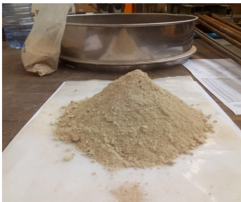
Figure 3.3. Waste paper sludge ash incinerated at 800°c.
