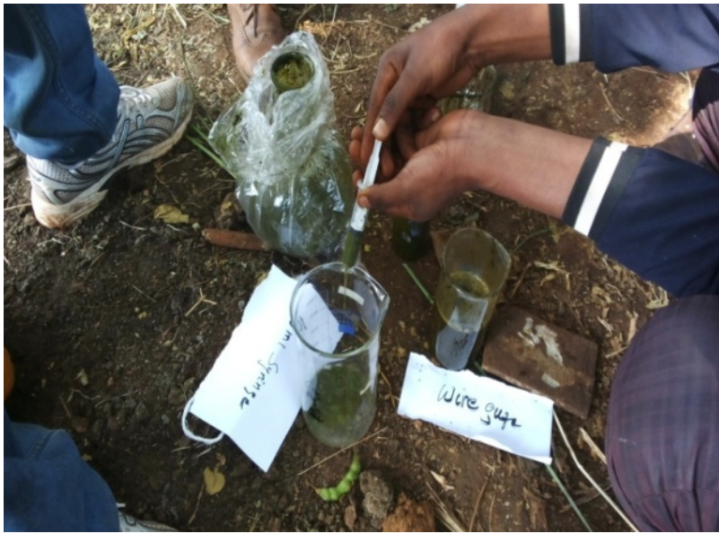
Plate 6.4. Filtering and measuring leaf extract
