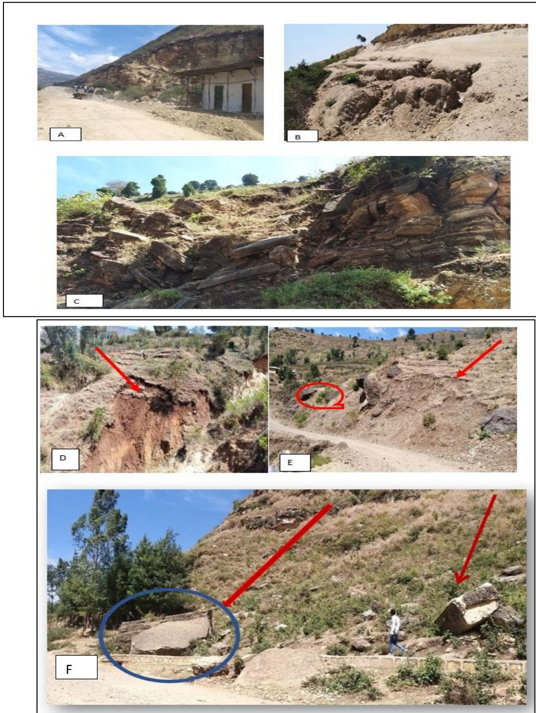
(A) Landslide along road cut near Funyan-Hujubo, (B) Soil cracks ready to slide at the side of road around Muhyadin Kabele, (C) Mixture of soil and rock slides near kundodo, (D) Mass of earth flow slide along river, (E) Rotational soil slides along a road and (F) Rock falls in around Funyan-hujubo
