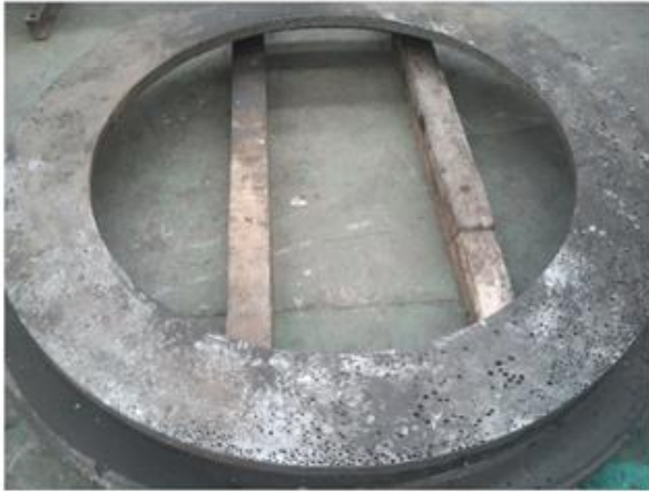
(a) Top surface of the defective drive disc
