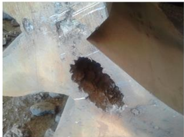
(f) Shrinkage cavity and sand sintering
