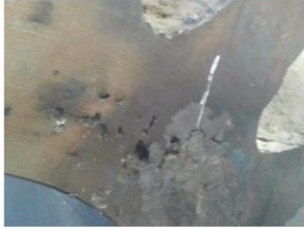
(b) Repaired shrinkage cavity
