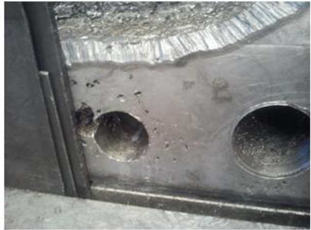
(b) Porosity on the surface of plate 4
