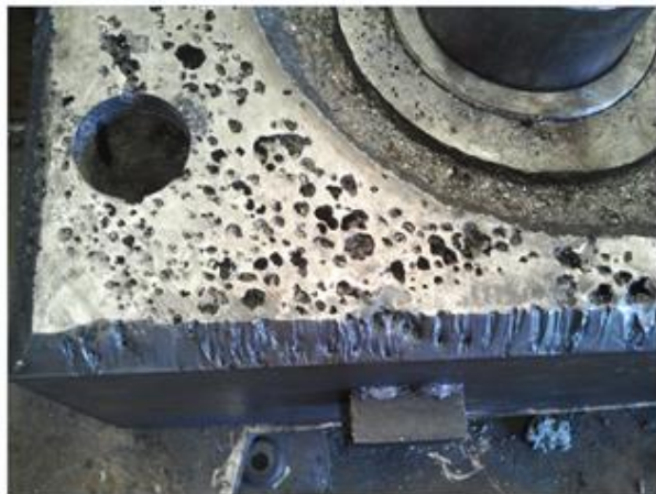
(c) Blow holes on plate 5
