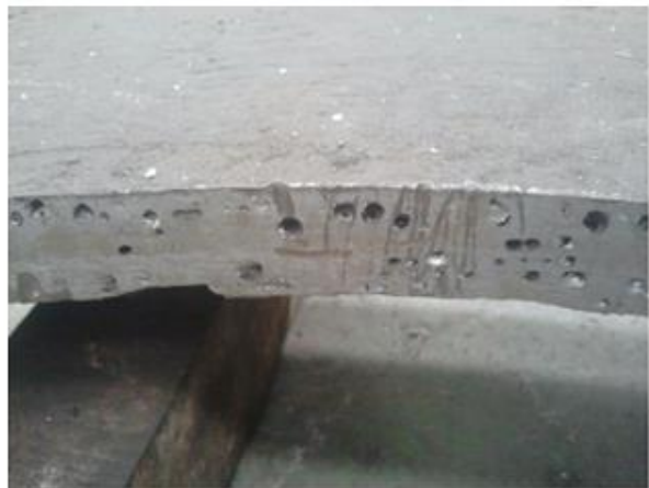
(f) Internal wall of the drive disc after first hand grinding
