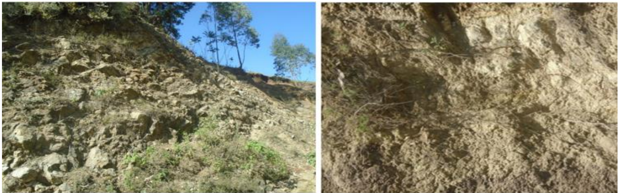
Figure 1. 9: Highly weathered gray to light gray color Unwelded tuff in the study area
