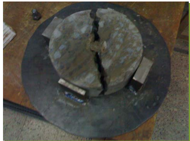
Fig. A.J-52 Ultimate Failure of a Plain Sample
