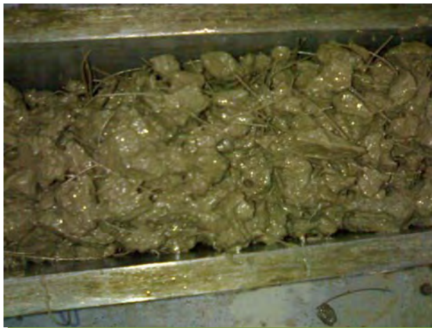
Fig. A.J-33 Steel Fibers in the Beam Mold
