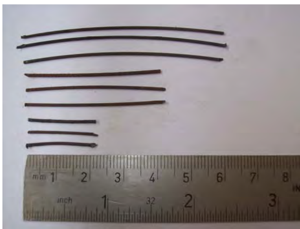
Fig. A.J-11 Steel fiber of different length
