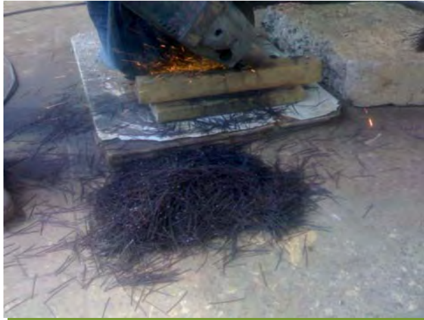
Fig. A.J-7 Cutting the Steel Fiber
