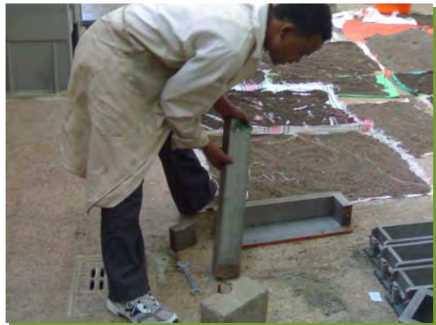
Fig. A.J-22 Assembling Beam Mould
