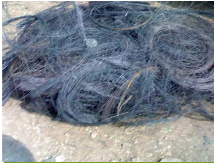
Fig. 4.1 Steel fibers (Bead wire) extracted from burnt tyres.
