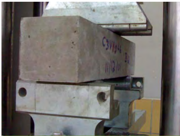
Fig. A.J-47 Two Point Loading Flexural Test
