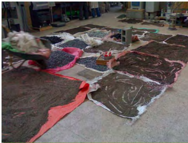
Fig. A.J-15 Drying the Aggregates
