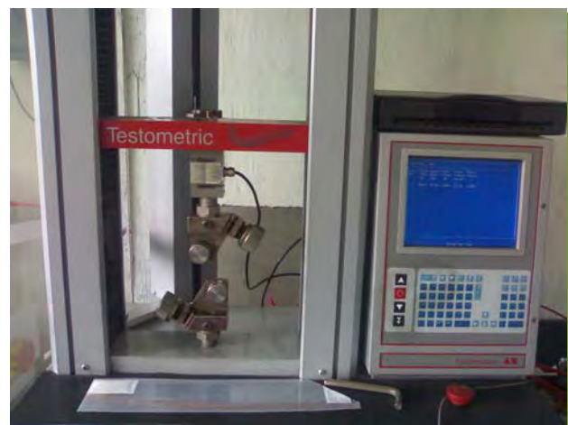
Fig. A.J-12 Test machine for tensile strength of steel fibers
