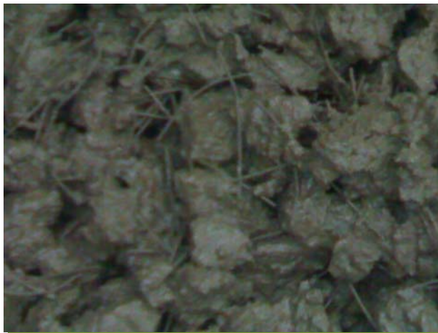
Fig. A.J-27 Distribution of Fibers in SFRC
