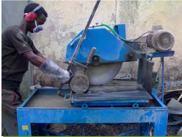
Fig. A.J-49 Cutting the Cylinder Samples
