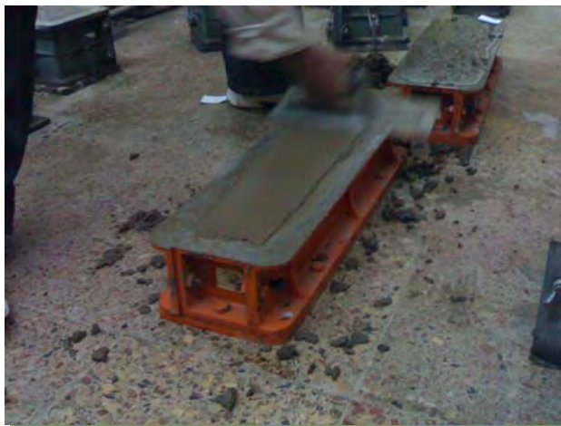
Fig. A.J-35 Trimming a Beam Sample
