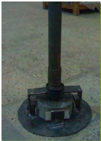
Fig. A.J-51 The Instrument for Impact test
