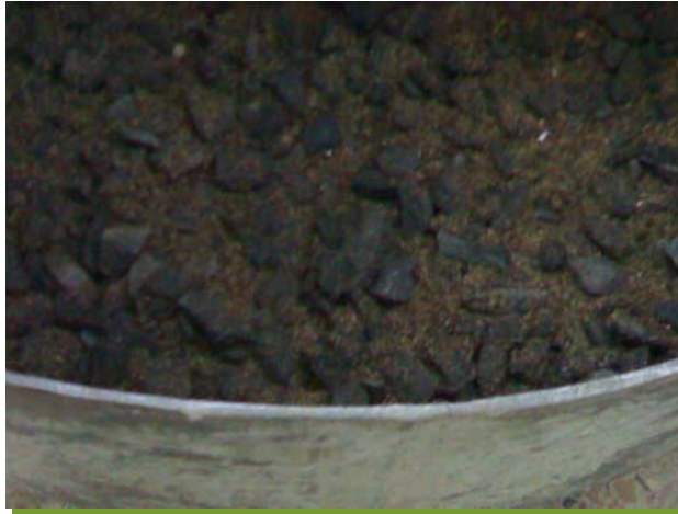
Fig. A.J-19 Bringing the Aggregates to SSD
