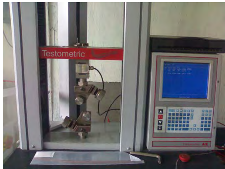
Fig. 4.4 Testometric Machine for tensile strength of steel fiber.
