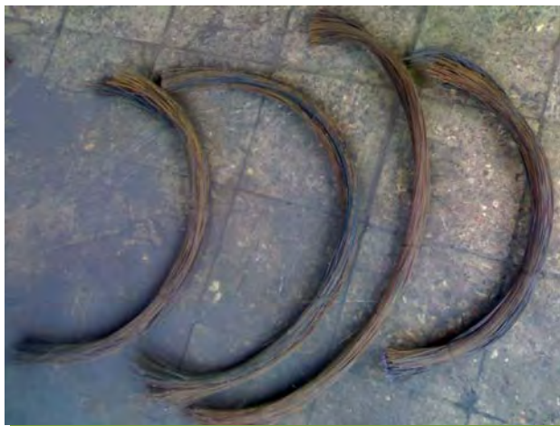
Fig. A.J-5 Steel fibers ready to be cut
