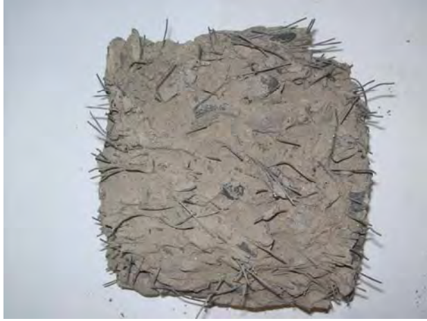
Fig. A.J-53 Distribution of steel fibers in a cube
