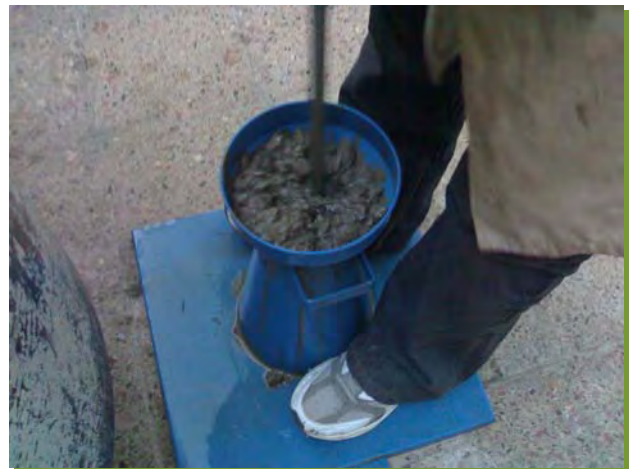
Fig. A.J-28 Preparing the Slump
