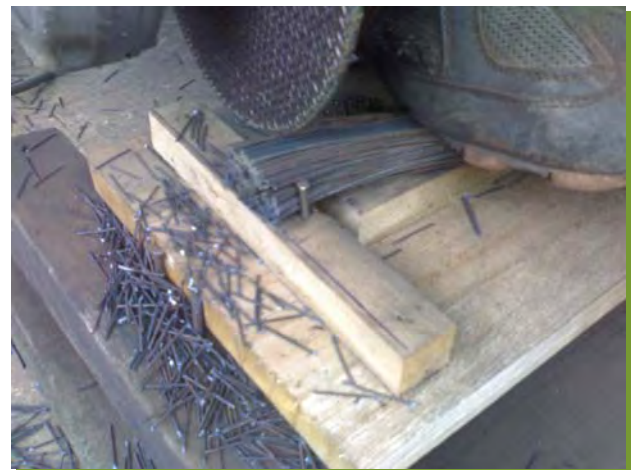
Fig. A.J-6 Cutting the Steel Fiber
