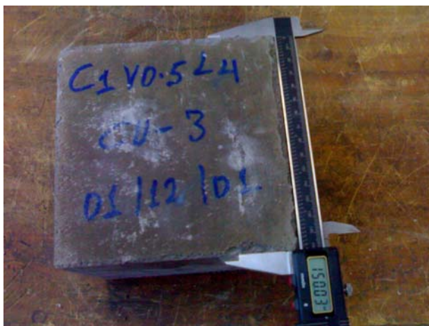
Fig. A.J-41 Measuring Dimension of a Cube
