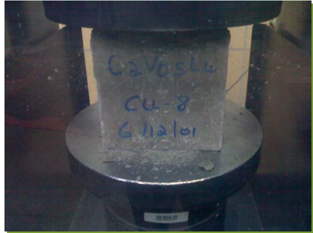
Fig. A.J-44 Crushing a Cube Sample
