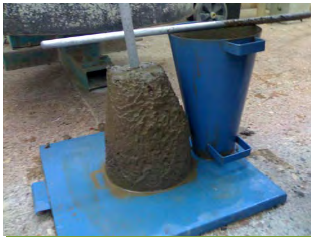
Fig. A.J-29 Slump for Plain Concrete
