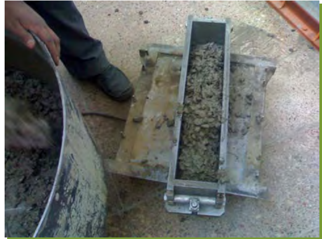
Fig. A.J-32 Casting a Beam Sample
