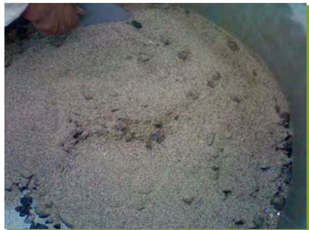
Fig. A.J-18 Bringing the Aggregates to SSD
