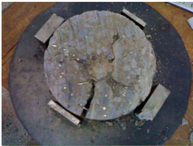
Fig. A.J-53 Ultimate Failure of SFRC Sample
