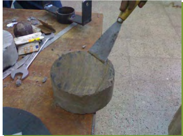
Fig. A.J-50 Greasing a sample for Impact test
