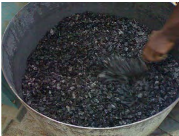
Fig. A.J-17 Water Adjustment for Coarse Agg.
