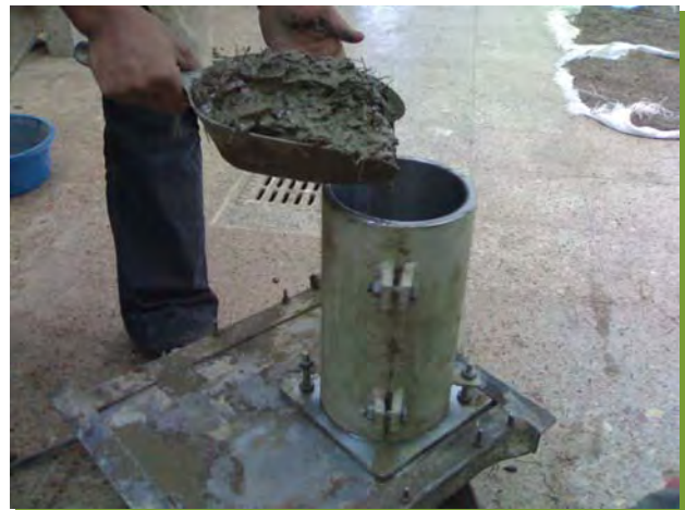
Fig. A.J-34 Casting a Cylinder Sample
