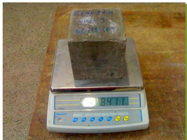
Fig. A.J-42 Weighing a Cube Sample
