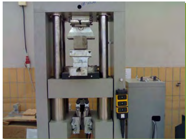
Fig. A.J-46 UTM Machine for Flexure Test
