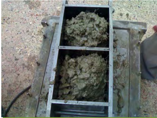
Fig. A.J-31 Casting Cube Samples
