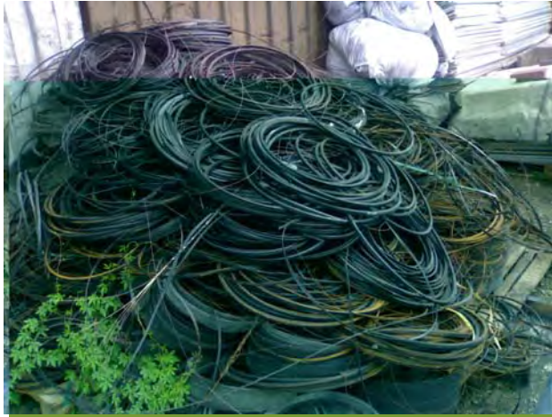
Fig. A.J-1 Defective Bead Wires to be Burn
