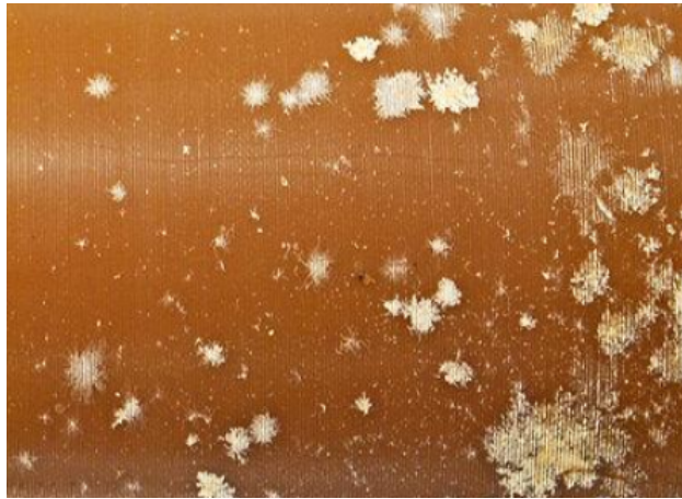
Figure 2.2: Degradation of brown wax cylinder
