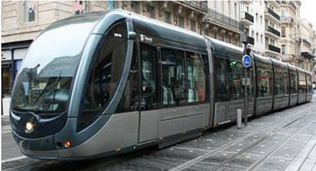
Figure 2.7. Alstom APS Underground Power for LRVs [10].
