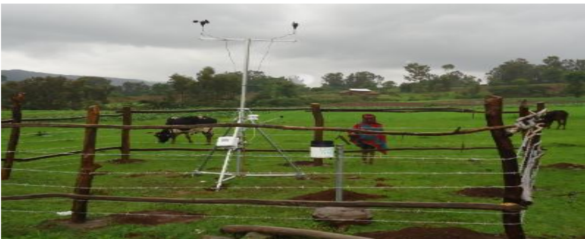
Figure 4 : Typical Automatic Weather station
