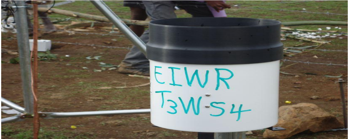
Figure 3: Typical tipping bucket type automatic rain gauge
