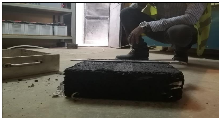
Figure 3-17 wheel truck specimen after test
