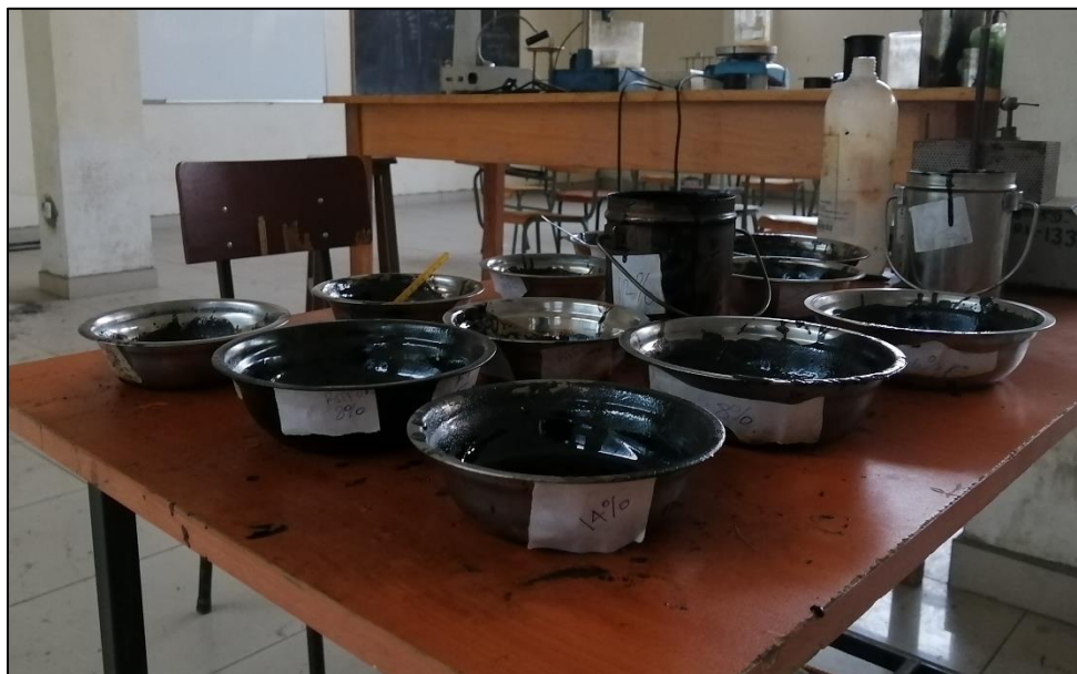
Figure 3-8 prepared samples with different asphalt and PVC proportion
