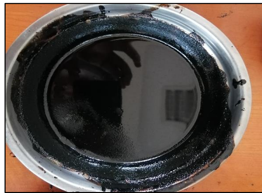
Figure 3-3 bitumen mixed with PVC powder
