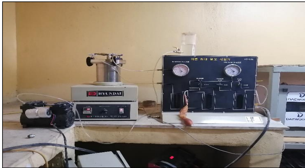
Figure 3-10 vacuum pump machine (used to suck the air in the asphalt mixture)
