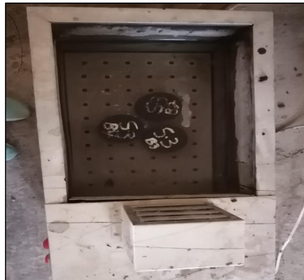
Figure 3-14 water bath for conditioning samples for moisture susceptibility test
