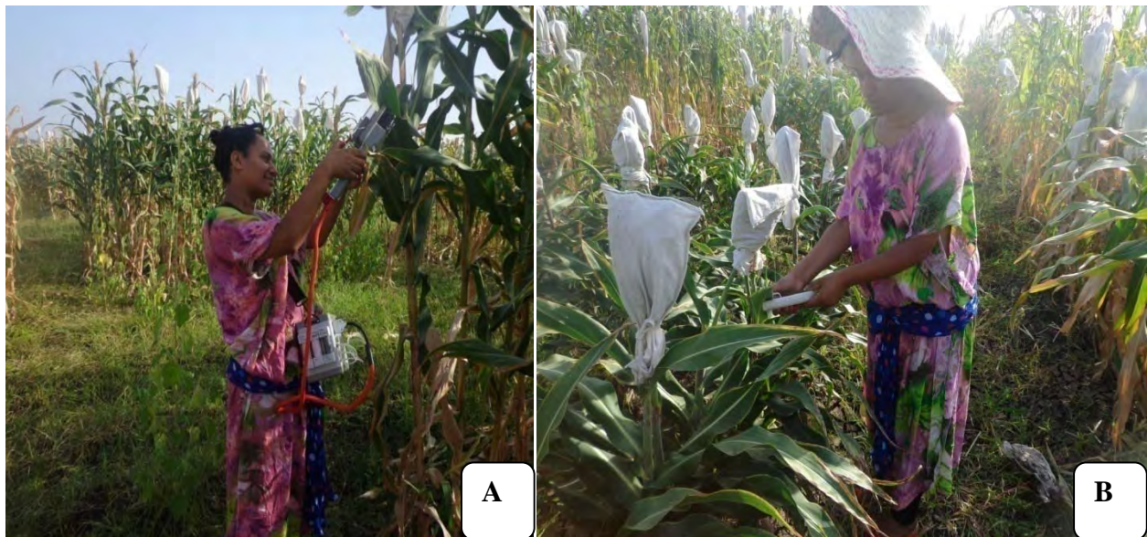
Figure. 3. (A) Measuring leaf gas exchange using Lc pro + photometer (B) Measuring chlorophyll content using chlorophyll content meter (CCM-200 pulse).
