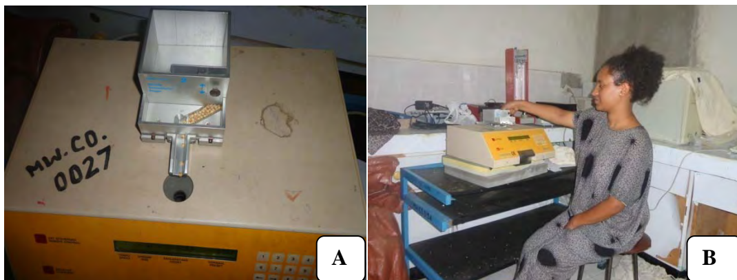
Figure.5. Seed counter machine (Contador Pfeuffer, German company) (A), Measuring 100 seed weight (B).
