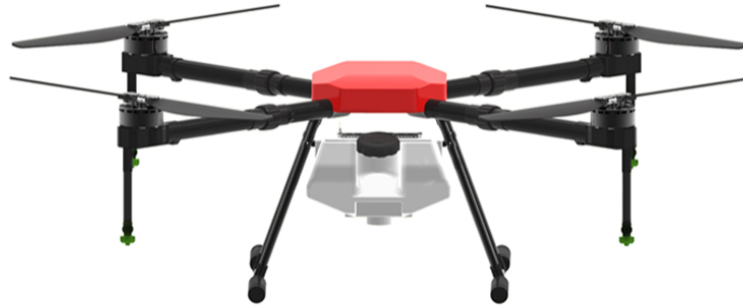
Figure 3.4: JMR-X1400: agricultural spray Quad-copter
