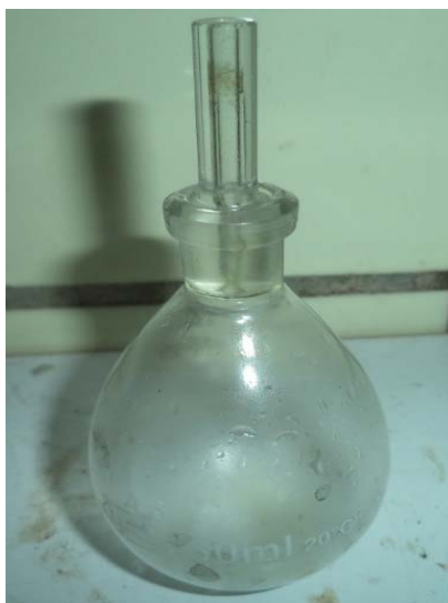
Figure 3.11: Pycnometer for specific gravity measurements (50mL, 20°C)
