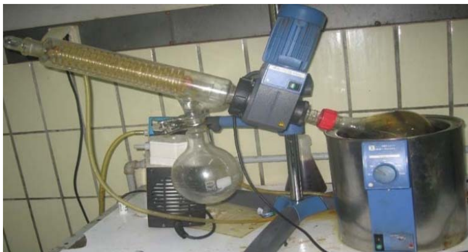
Figure 3.9: Distillation for purification of ethanol
