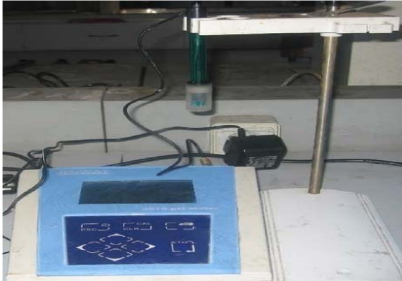
Figure 3.6: pH meter for neutralization of hydrolysates solutions
