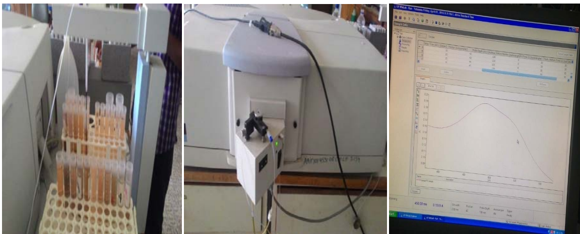
E6: Total reducing sugar analysis using UV Spectrophotometer
