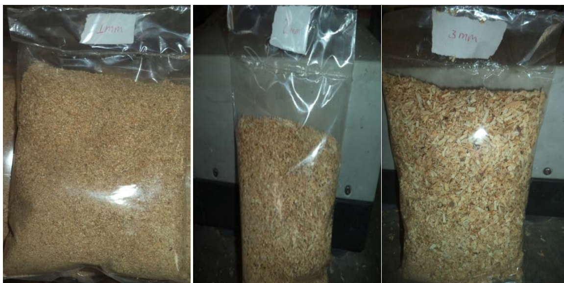
Figure 3.2: Sample prepared in different particle sizes (a) 1mm, (b) 2mm and (c) 3mm
