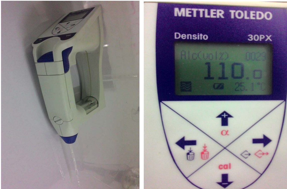
Figure 3.10: Alcoholmeter for ethanol content measurement
