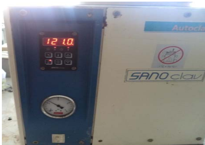
Figure 3.7: Autoclave reactor heater used for sterilization
