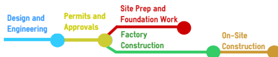
Figure 5.34: Convention Vs Modular Construction Timeline Comparison
