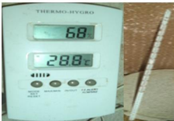
Plate 5.1. Thermo-Hygro and thermometer follows Relative Humidity and Temperature
