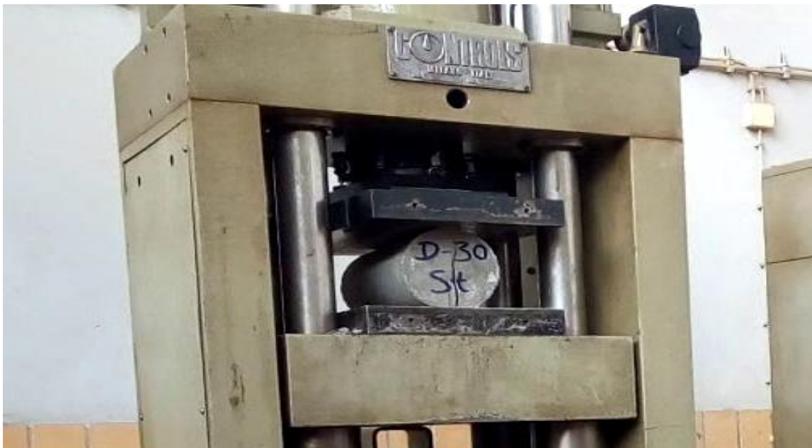
Figure 3-5: Concrete split tensile strength test machine
