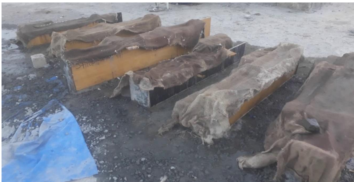
Figure 3-10: Curing of concrete on beam specimens, cubes and cylinders
