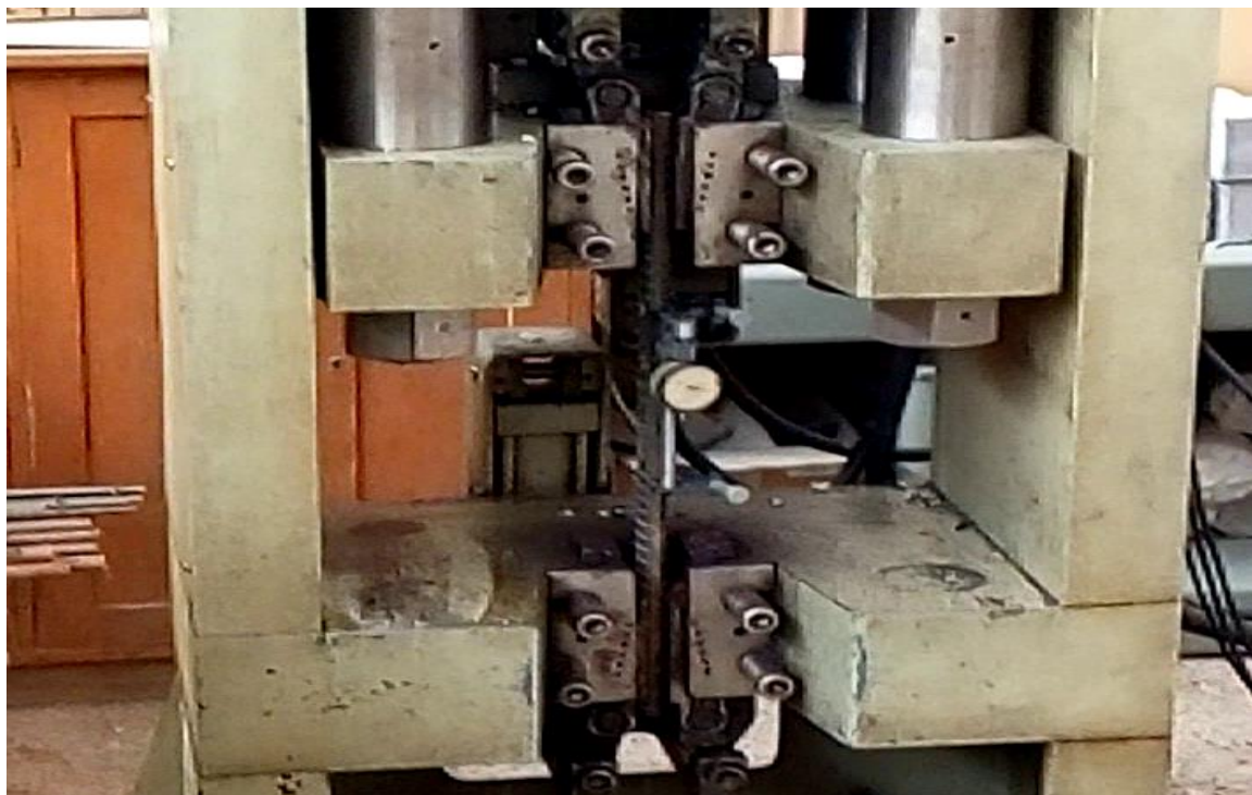
Figure 3-6: Universal Testing Machine testing tensile strength of reinforcement bar
