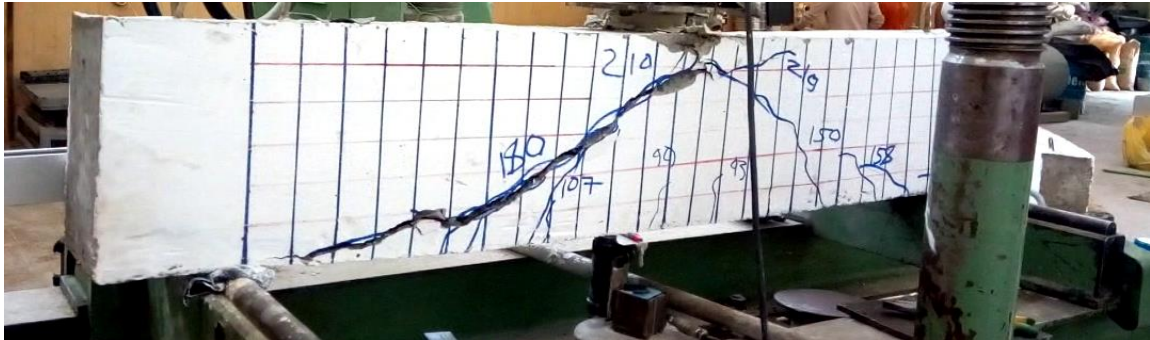
Figure 5-5: Specimen BS30 beam with shear reinforcement after failure
