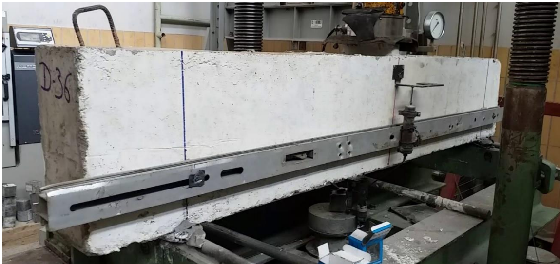
Figure 3-16: Displacement measuring device installed at the back of the specimen
