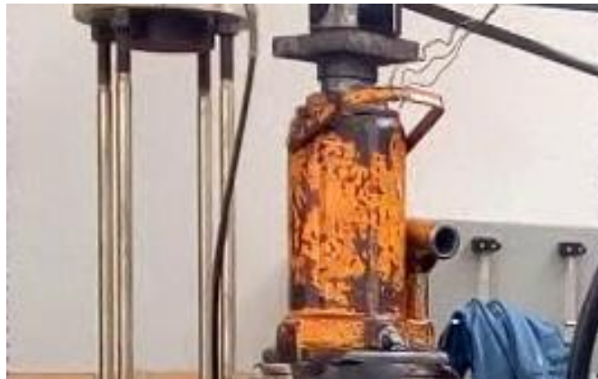
Figure 3-14: Manual hydraulic jack with maximum capacity of 300KN
