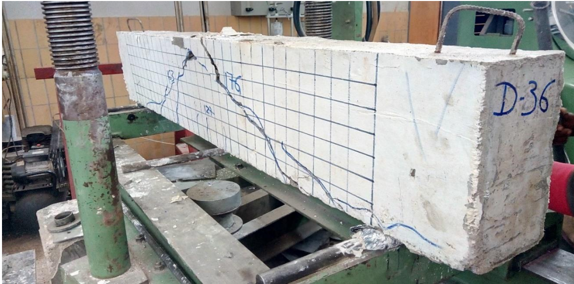
Figure 5-3: Specimen B36 beam without shear reinforcement after failure
