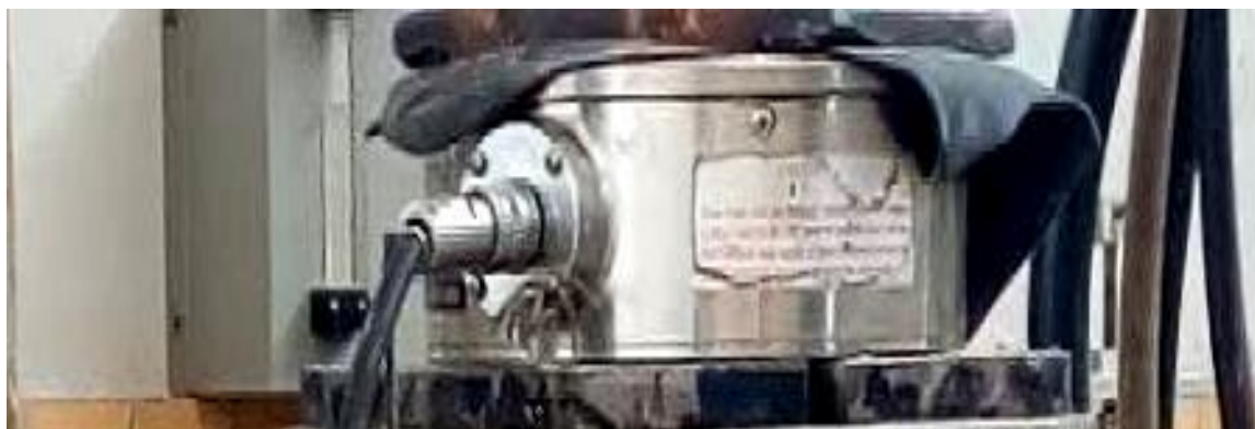
Figure 3-13: Loading cell used to read applied load
