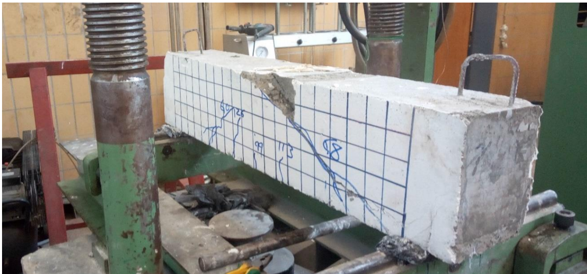
Figure 5-1: Specimen B24 beam without shear reinforcement after failure
