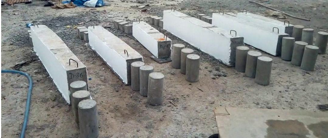
Figure 3-11: Beam specimens painted white on both faces before test
