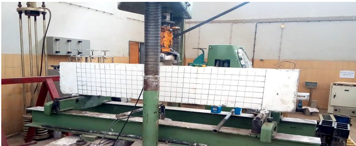
Figure 3-12: Loading setup during testing of beam specimen
