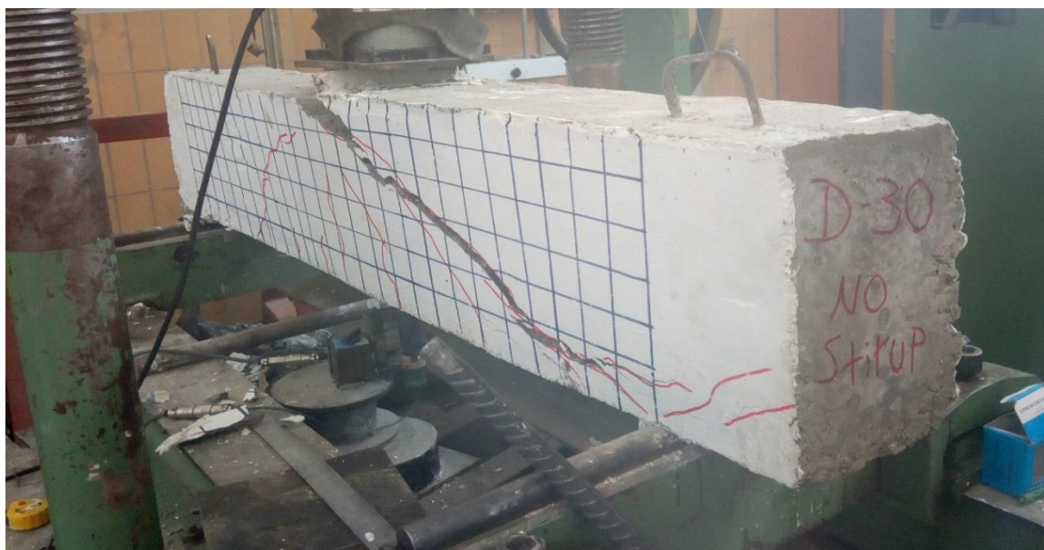
Figure 5-2: Specimen B30 beam without shear reinforcement after failure
