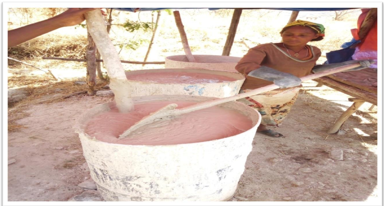
Figure 3.19. A woman boiling the lime powder, which was buried, with water (Photo by Kedir 2018)
