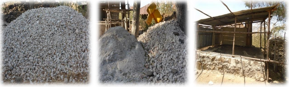
Figure 3.55 Conservation Process of Bahri Ginb, coarser lime stone (the left two figures) and the buried lime powder (right figure) (Photo by Kedir 2018)
