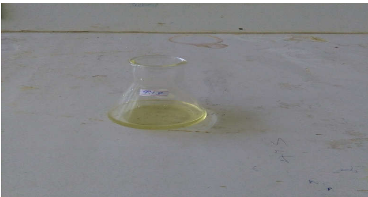
Figure 7: Pale yellow color left when nearly all iodine has reacted with thiosulfate during titration
