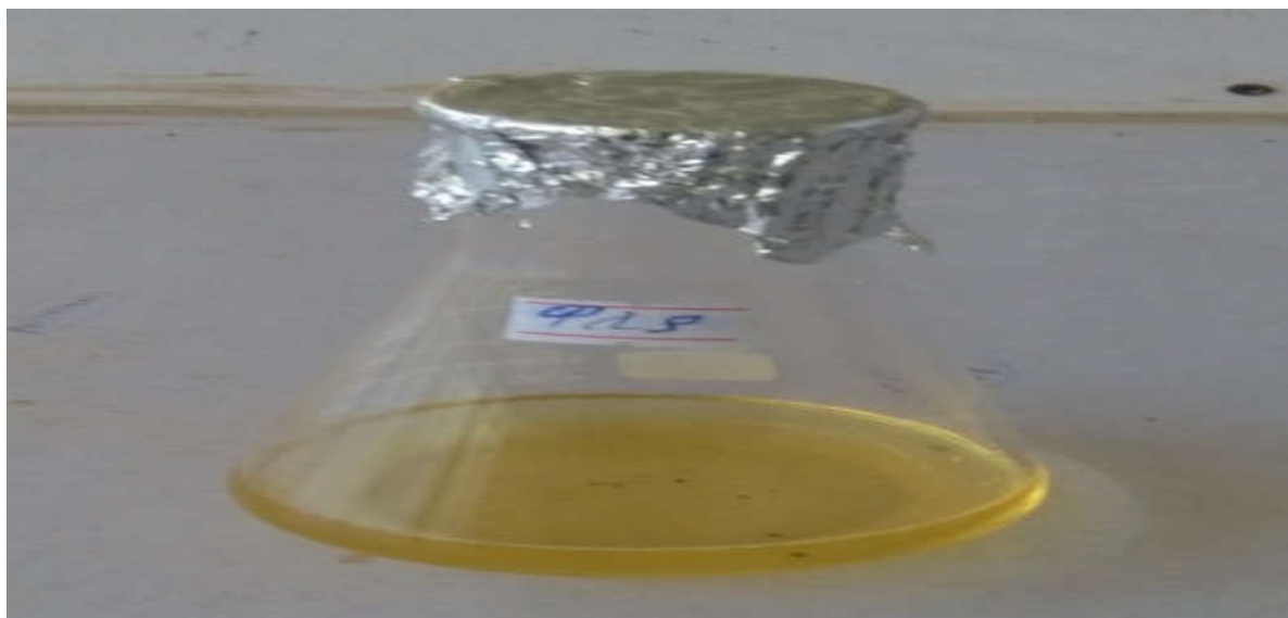
Figure 6: Yellow color of iodine formed from the reaction of iodized salt with acidic iodide solution
