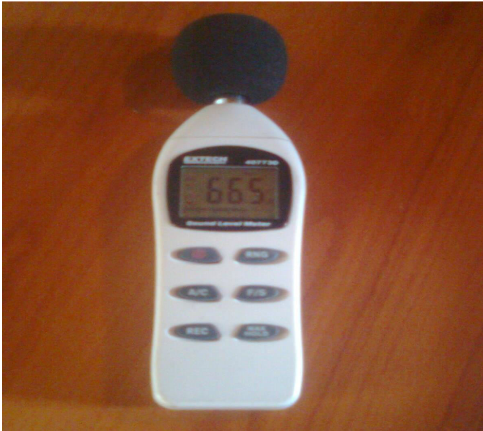
Picture 14-The Extech 407730 Digital Sound level Meter (Photo by the author-18/05/2014)
