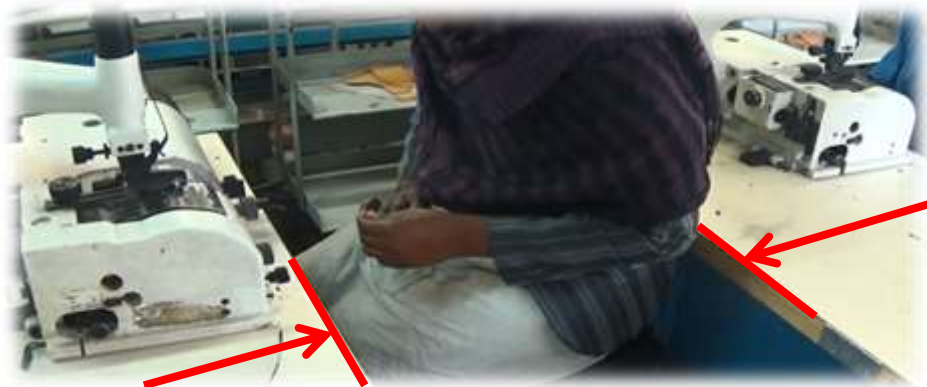
Figure 4.4:- Not enough space between stitching machines (Source: Field visit)
