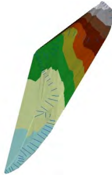
Figure 4.30: Generated water surface TIN
