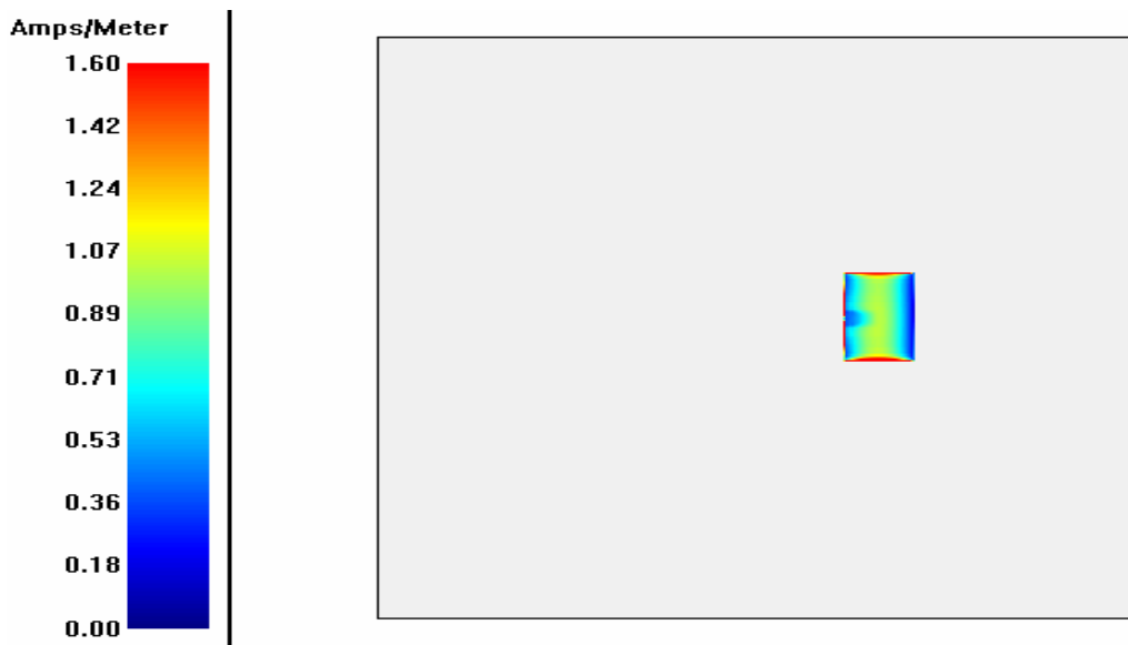
Figure 5. 12 The current density diagram of proximity coupled at 3.485GHz
