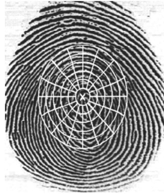
Figure 2.21 Reference point (x), the region of interest, and 80 sectors superimposed on a fingerprint [8].
