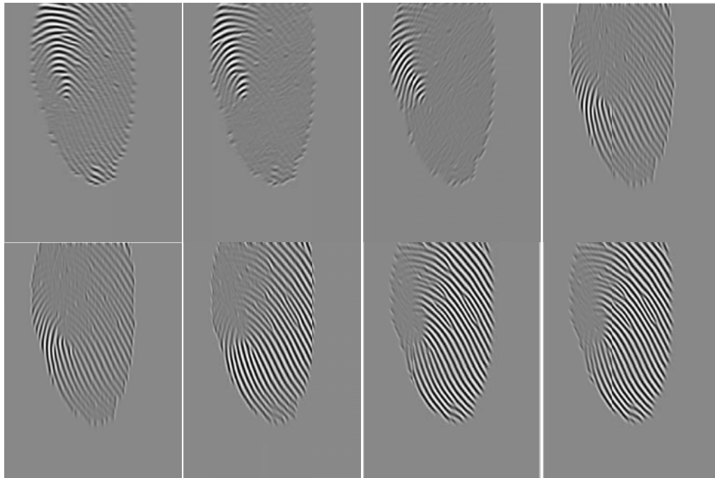
Figure 3.8 the filtered images of the input image shown in figure 3.2 in 8 different directions by Gabor filter.
