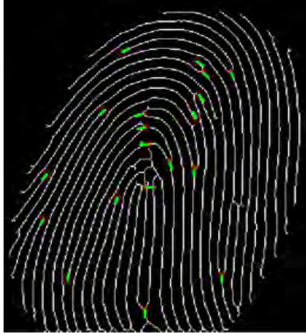
Figure 2.15 Extracted minutiae of the enhanced image shown in figure 2.13.
