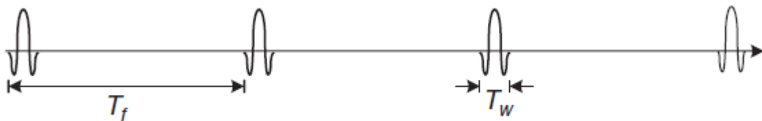
Figure 2.5: A sequence of second order Gaussian pulse train with low duty cycle
