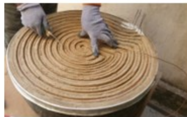
d) Placing of one copper wire circuit in grooves
