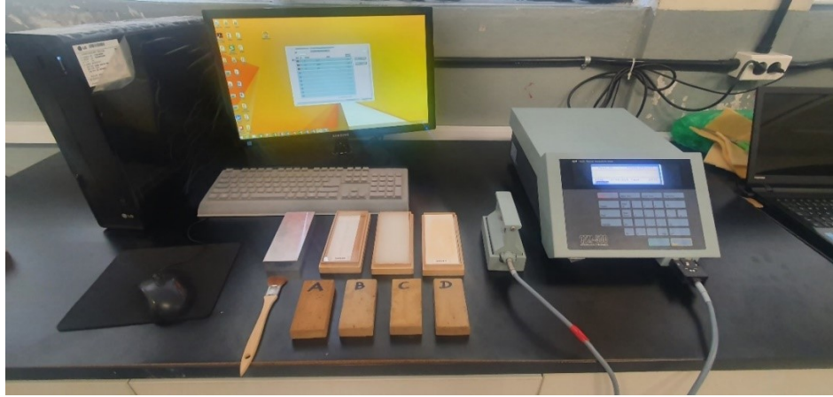
Figure 3-13. The QTM- 500 and thermal conductivity measuring experimental setup
