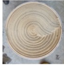
b) One heating element circuit placed in grooves
