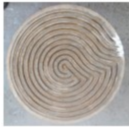
c) Double heating element circuit placed and sealed
