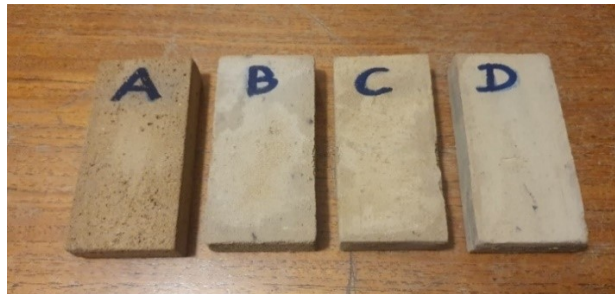
Figure 3-12. Clay plate samples for a thermal conductivity test.
