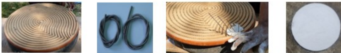
a) Grooved clay plate b) Heating element c) Heating element placed d) Sealed clay plate
