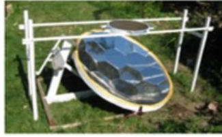
a) Prototype solar fryer, (Gallagher, 2011).
