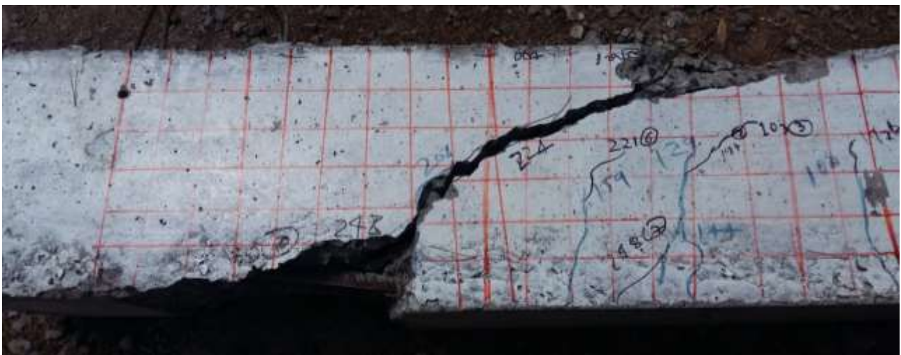
Figure 5.6 : B2C90 after failure (half view)
