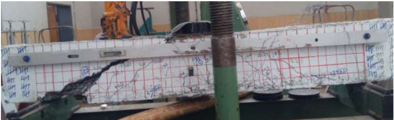
Figure 5.8 : B2C85 after failure
