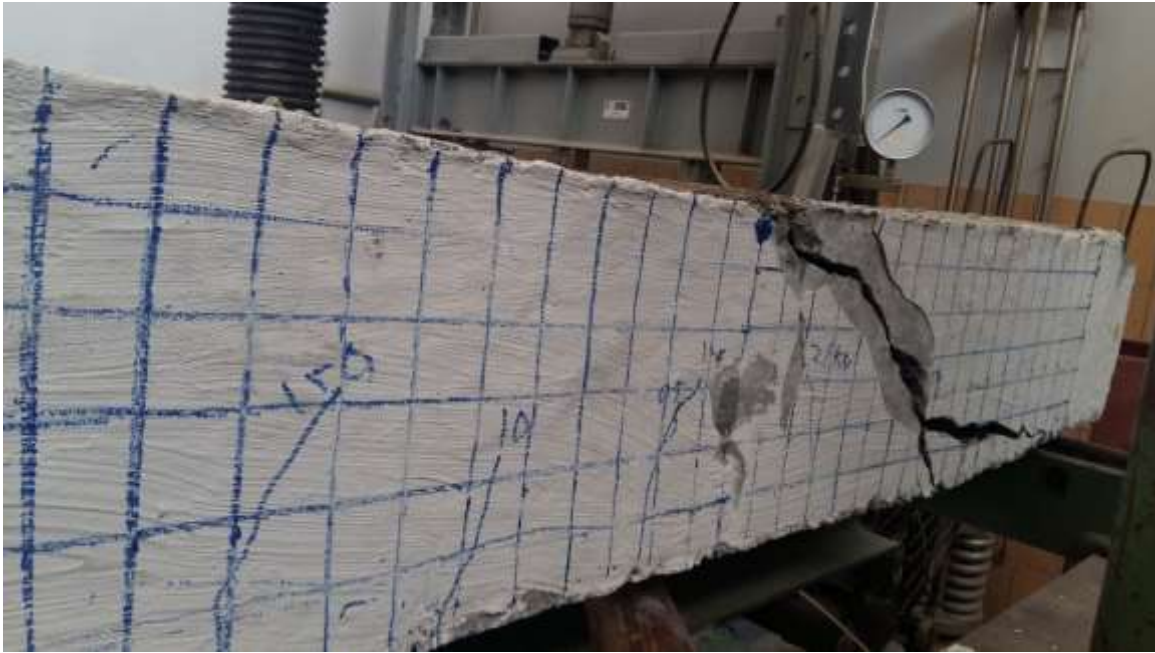
Figure 5.2 :B1M after failure
