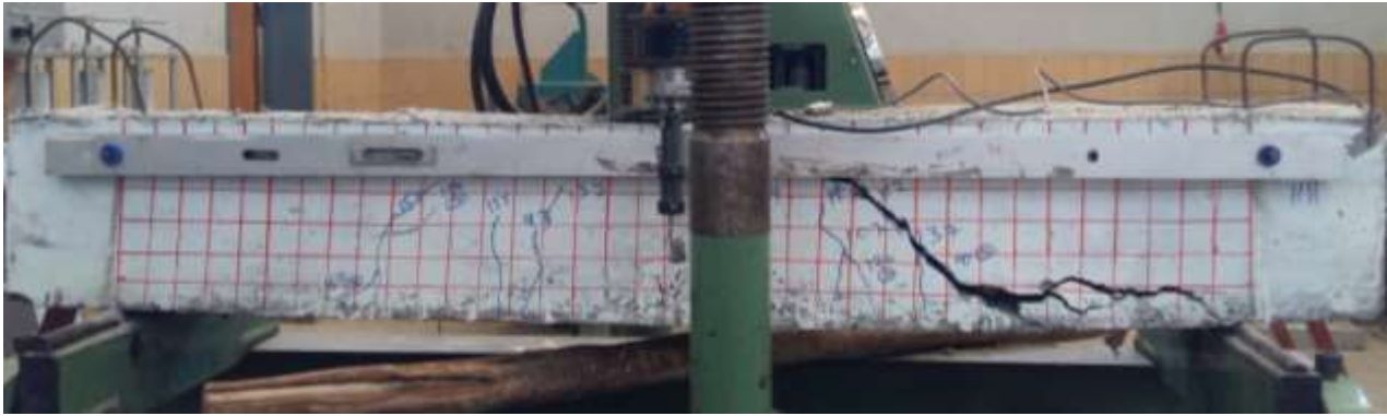
Figure 5.3 : B1C90 after failure
