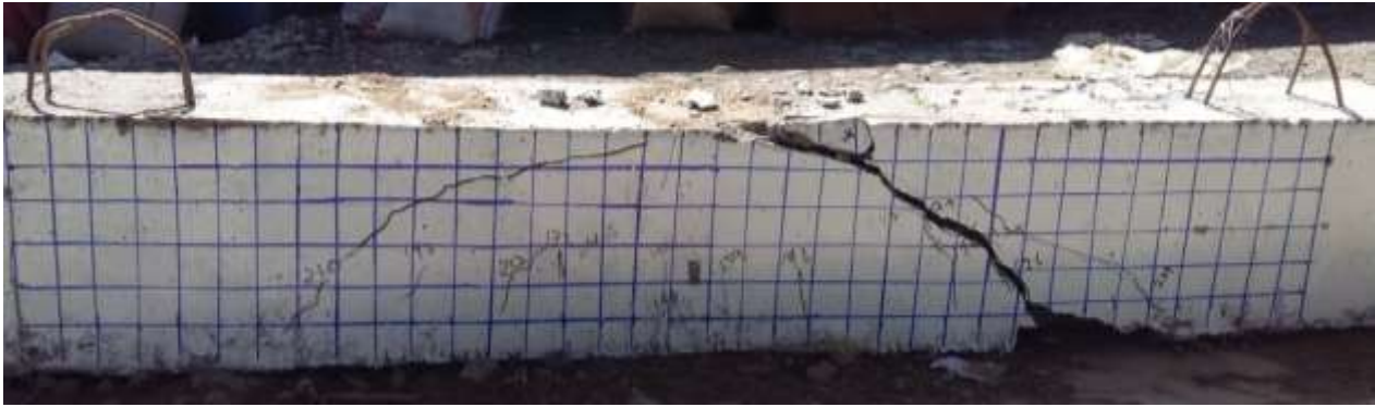
Figure 5.4 : B2M after failure
