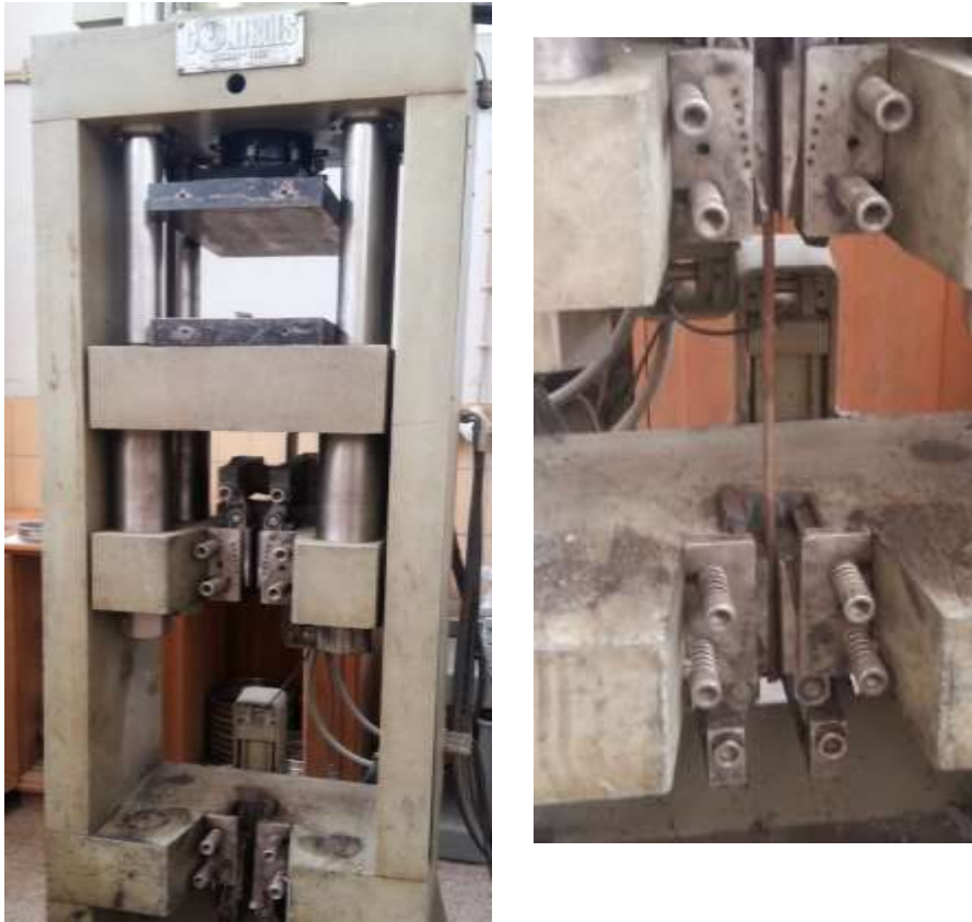
Figure 3.6 : Tension test performed on Rebar
