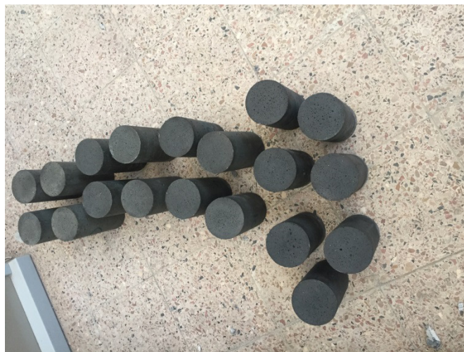
Picture 5: cylindrical cubes contains bagasse ash
