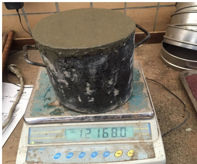
Picture 4: Wet density determination using known container volume
