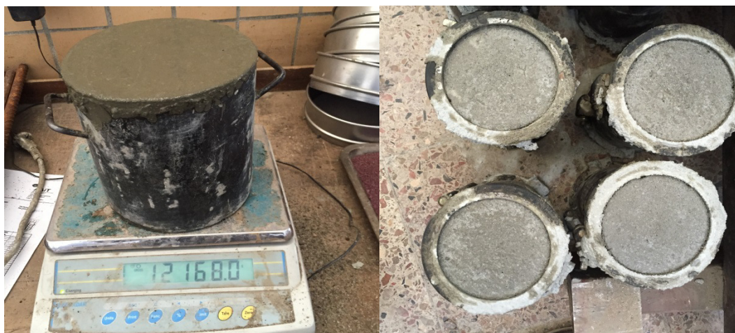
Figure 6: Bleeding of mortar during measurement of wet density and its effect on plastic shrinkage.
