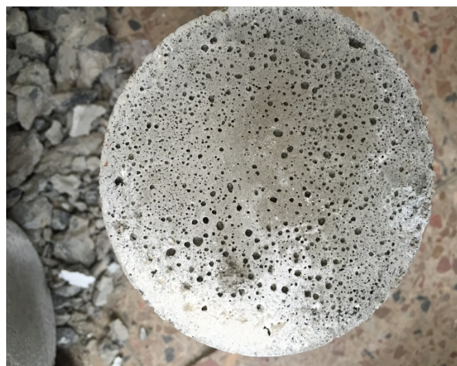
Picture 3: Formation of air bubbles inside the mortar
