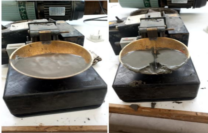
Figure 3-10: Liquid limit determination for pozzolanic sand
