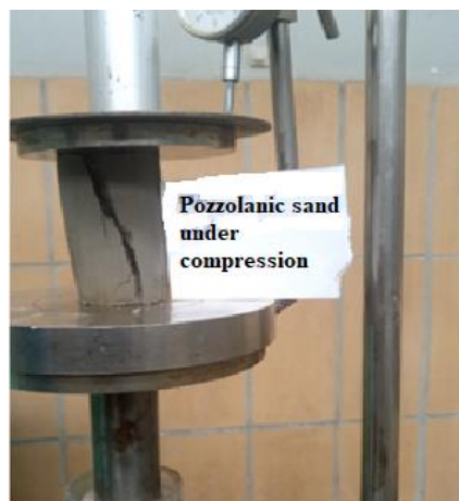
Figure 3-12: Pozzolanic sand under compression
