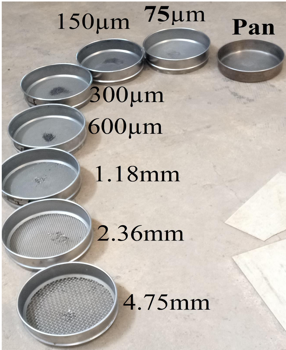
E-1: Sieve Analysis and samples retained on each sieve
