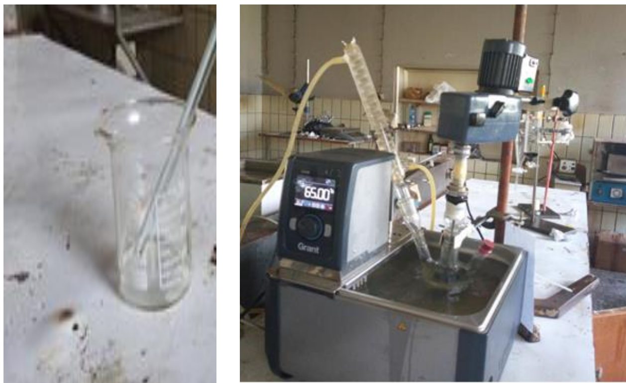
Figure 3.6 Mixing of NaOH and methanol and experimental transesterification reaction process
