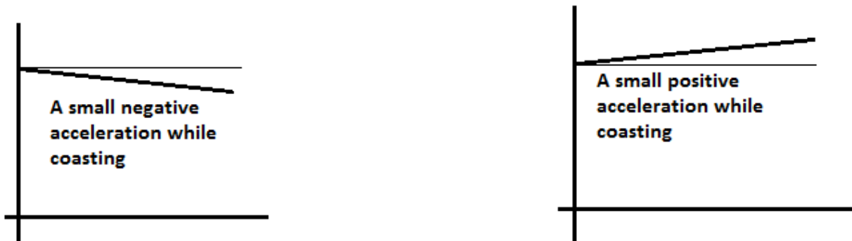
Figure 4.11: A small acceleration or deceleration rate of coasting regime can be approximated by a cruising regime.
