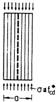
Fig 3.31 prismatic strut stress distribution
