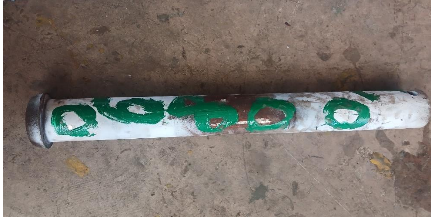
Figure 7: Cracked knuckle pin
