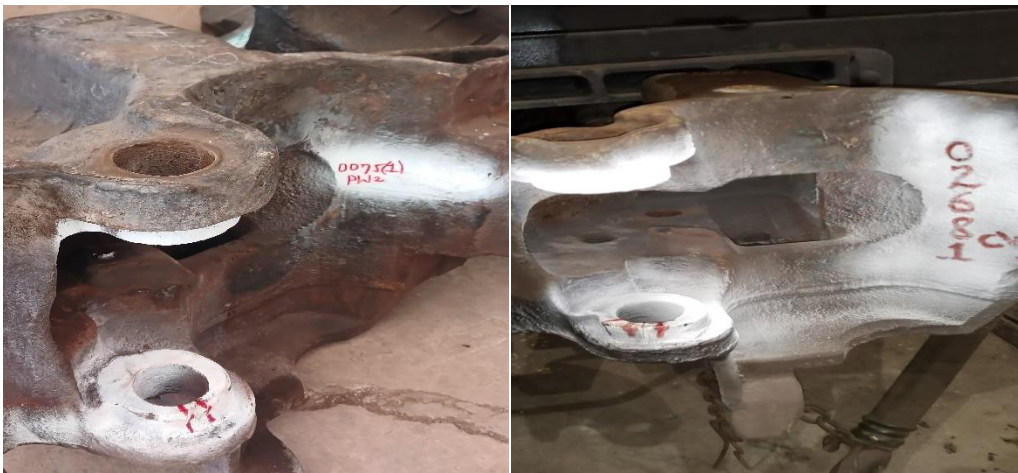
Figure 6: Cracked coupler head
