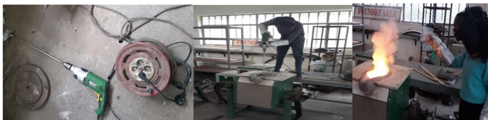
d) Adding salt and pure magnesium into the composite and removing the slag Stirring the reinforcement with the molten alloy by stainless steel stirrer
