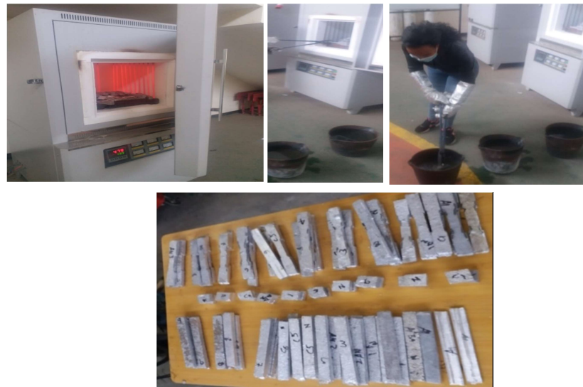
Figure.3.11: Heat treatment, quenching of the specimen, and test specimens
