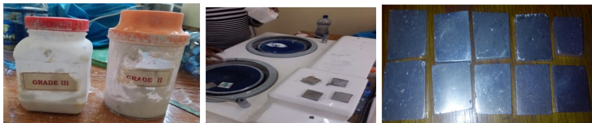
Figure.3.16: a) Grade II & III Polishing gel b) MP-2B Grinder Polisher c) the final specimens for test
