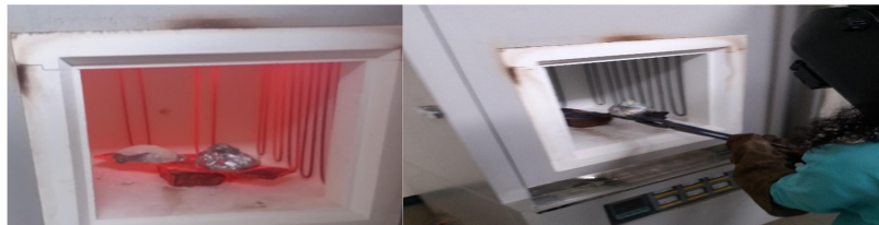
b) Preheating the reinforcement in heat treatment furnace
