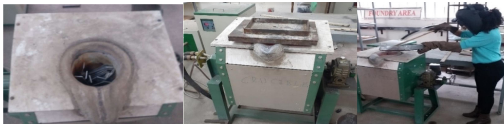
c) Mixing the reinforcement into molten aluminum alloy
