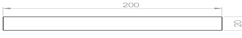
Figure 3.7: flexural test specimens as ASTM E290
