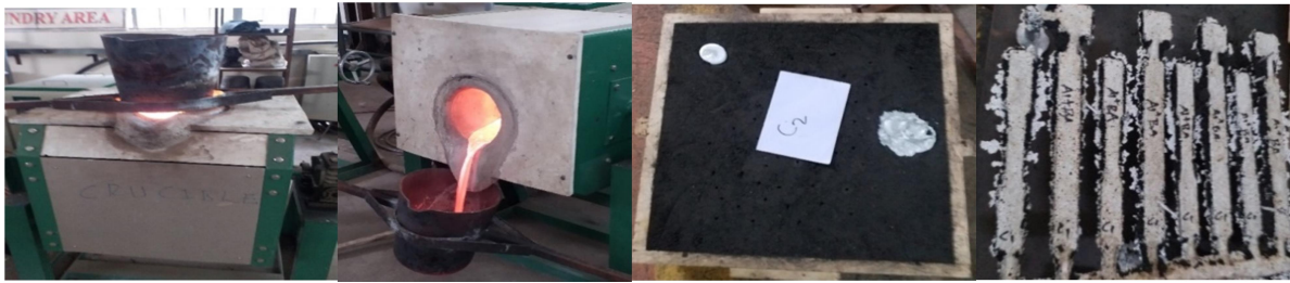
e) Pouring the molten composite into the mold and removed after 3hr
