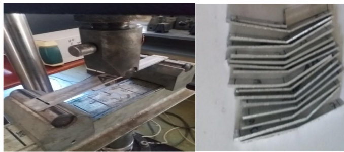
Figure 3.14: (a) Typical specimen under bending test on UTM, (b) Specimens after the test
